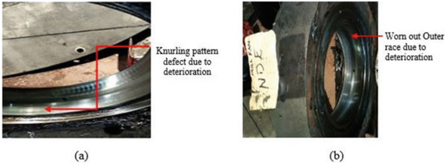
Fig. 3 a Knurling pattern defect identified on motor drive end side bearing and b normal wears on outer race due to deterioration on non-drive end
