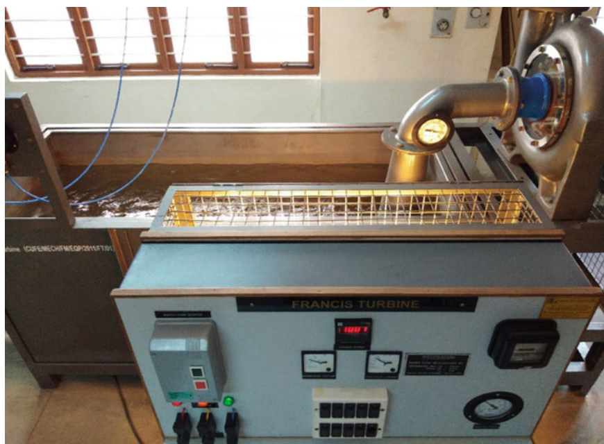
Fig. 1 Experimental setup of hydro turbine-generator unit
