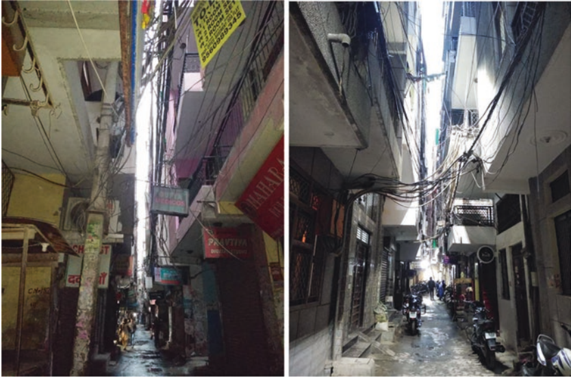
Fig. 16.1 (a) Commercial Establishments found in residential premises in Munirka. Such mixed land use is common in Lal Dora areas. (b) High Vulnerability due to low hanging high voltage electric wires and five-story vertical building constructions in Munirka village. (Source: Author's)
