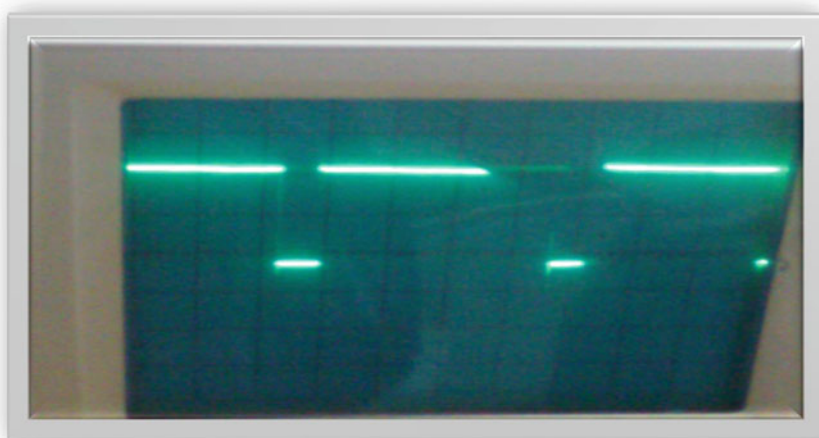
Fig. 12 PWM pulses for converter (switch 1, 3)
