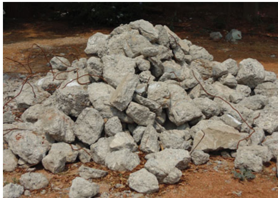
Fig. 3 Demolished concrete material
