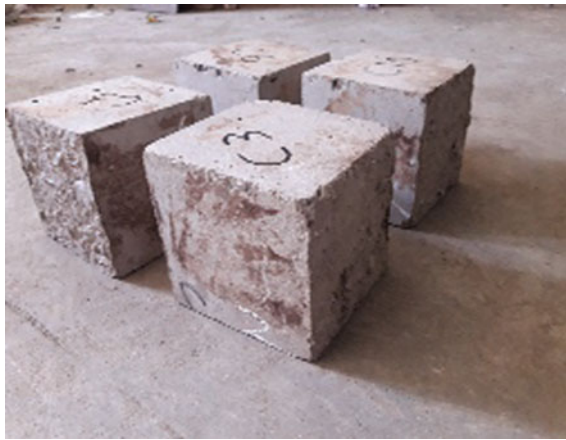
Fig. 4 Concrete incorporated with alumina silicates samples subjected to elevated temperature
