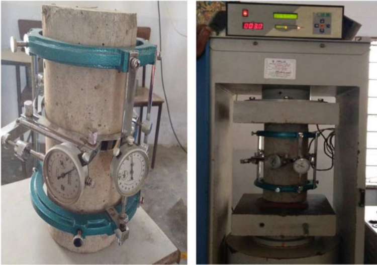
Fig. 1 Arrangement of the dial gauges for the elastic properties of SFSCC and testing setup
