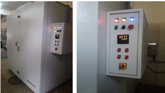
Fig. 3 Heavy-duty ovens used for subjecting the cubes to elevated temperature
