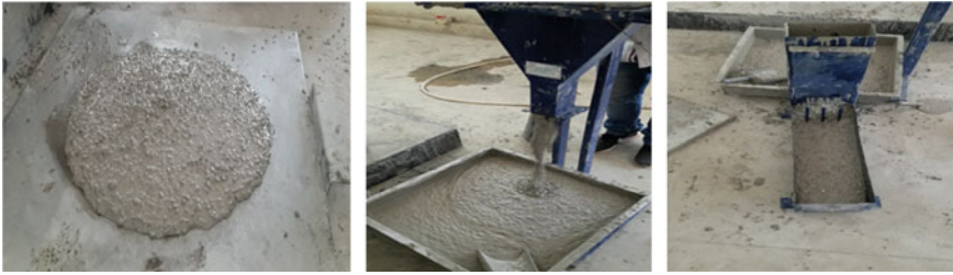
Fig. 2 Details of slump flow, V-funnel and L-box test
