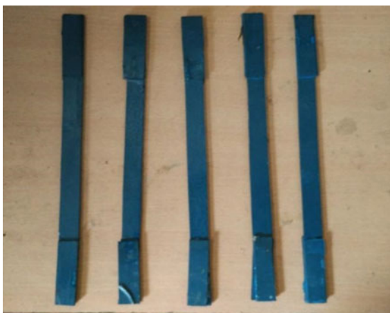
Fig. 15 Samples of 0.5 wt% MWCNTs before test
