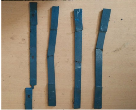
Fig. 16 Samples of 0.5 wt% MWCNTs after test
