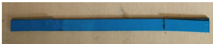
Fig. 10 Specimen for tensile testing
