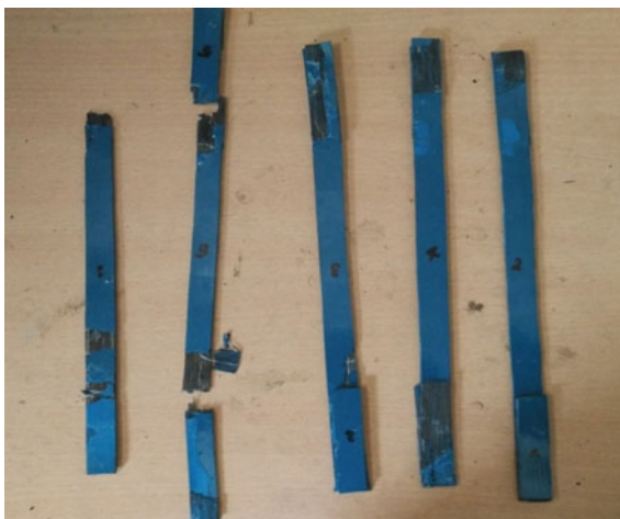
Fig. 14 Samples of 0.2 wt% after test
