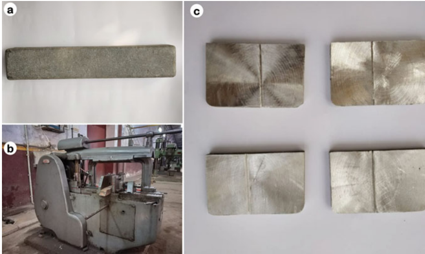
Fig. 1 Preparation of magnesium specimen from magnesium billet
