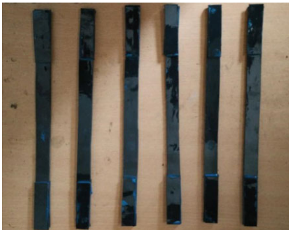
Fig. 17 Samples of 0.5 wt% MWCNTs before test
