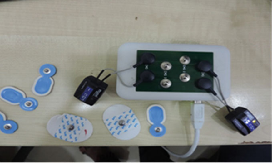
Fig. 1 The myon-aktos-mini wireless data acquisition system
