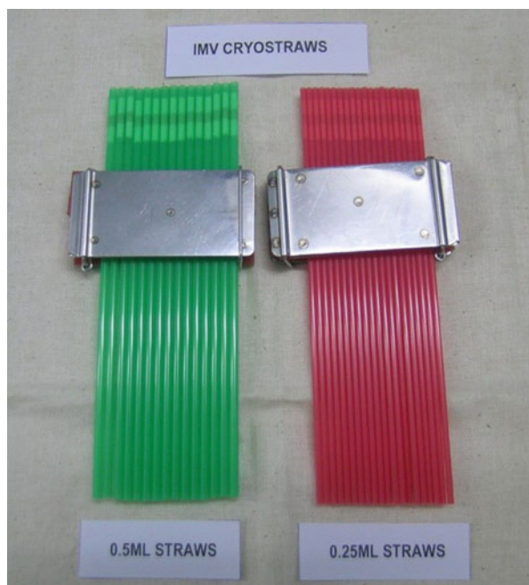
Fig. 7.4 IMV cryostraws of 0.25 mL and 0.5 mL volume (Photo courtesy: J. Stephen Sampath Kumar)
