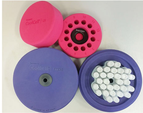
Fig. 12.6 Equipment for slow-rate freezing. Example of commercially available freezer boxes to ensure a cooling rate of -1\text{ }^{\circ}\text{C}/\text{min} in a -80\text{ }^{\circ}\text{C} freezer, allowing grams of the gonadal tissue to be cryopreserved
