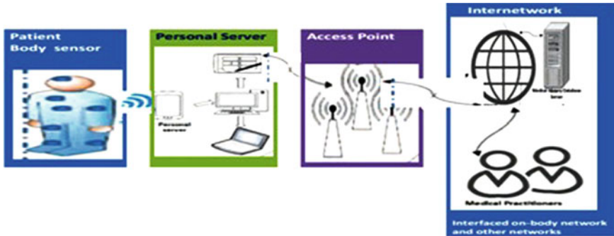
Fig. 2 Architecture of on-body communication network [5]
