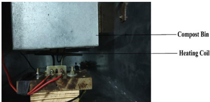
Fig. 7 Heating section of the kitchen waste recycler bin
