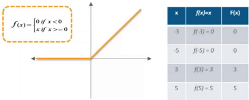
Fig. 4 ReLU function is half rectified. f(x) is zero when x is less than zero and f(x) is equal to x when x is above or equal to zero
