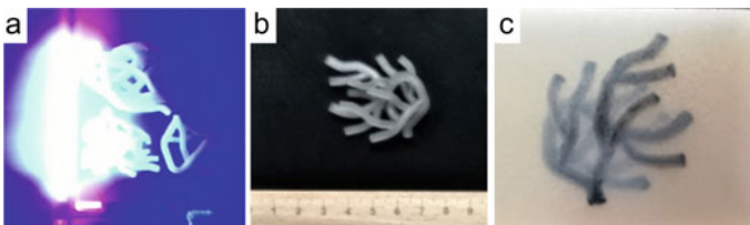
Fig. 4 Phantom manufacturing. a 3D printing process. b Final model. c Final phantom in agar
