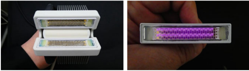
Fig. 13 Photograph of LED-based PAUS probe in which two LED arrays (750/850 nm) are placed on both sides of a linear array US probe (7 MHz) (left). Photograph of the LED array (right) with four rows of LED elements in which row 1 and 3 are 850 nm elements, row 2 and 4 are 750 nm elements. In this picture, 850 nm elements are activated and captured using an IR camera [Reprinted with permission from 44]
