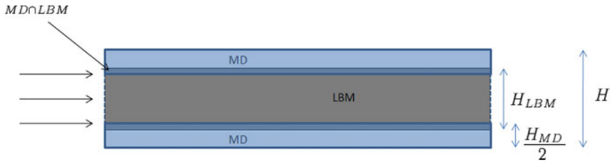
Fig. 6.8 Schematic of LBM-MD coupling in a planar channel (Marsh 2010)
