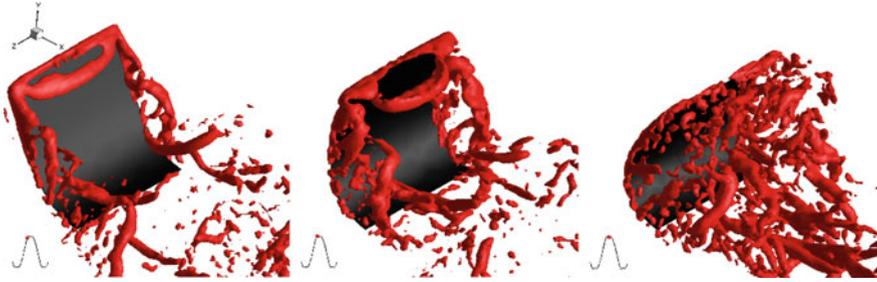
**Fig. 4.6** Snapshots of Q-criterion iso-surfaces (Hunt et al. 1988) at three time instants showing the inverted flag near the maximum ( $y_{\max}$ ) deflection. These snapshots elucidate the 3D coherent structures in the wake of the flapping flag. The red dot in the inset of each figure identifies the corresponding instant. Figures reprinted with permission from Gilmanov et al., *Journal of Computational Physics*, 300, 814–843 (2015). Copyright 2015, American Institute of Physics
