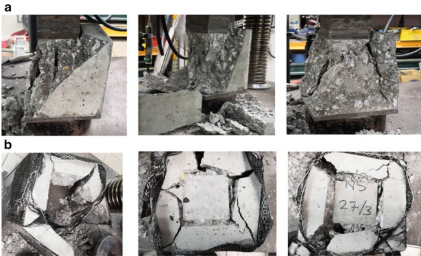
Fig. 5 a Failure mode for unwrapped concrete block. b Failure mode for CFRP wrapped block
