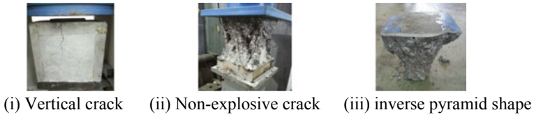
Fig. 4 Modes of failures for unreinforced concrete blocks
