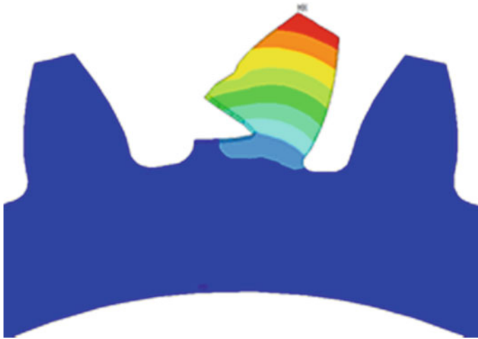
Fig. 5 Cracked tooth of gear
