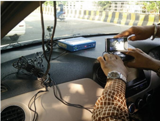
Fig. 6 Setting up of V-BOX
