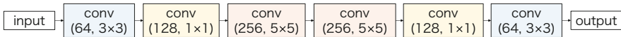
Fig. 7.5 An example of a genotype and a phenotype of CGP-CAE. A phenotype is a graph representation of a network architecture and a genotype encodes a phenotype. They encode only the encoder part of a CAE and its decoder part is automatically created such that it is symmetrical to the encoder part. In this example, the phenotype is defined on a grid of three rows and three columns
