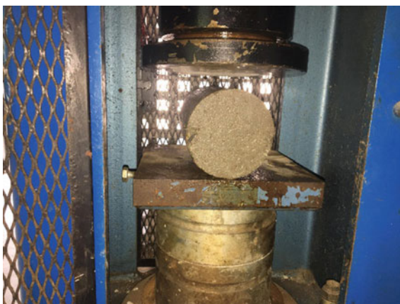
Fig. 2 Sample for splitting test of coconut fibre-reinforced cement (CFRC) concrete
