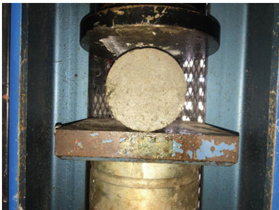
Fig. 1 Sample for splitting test of plain cement concrete (PCC)
