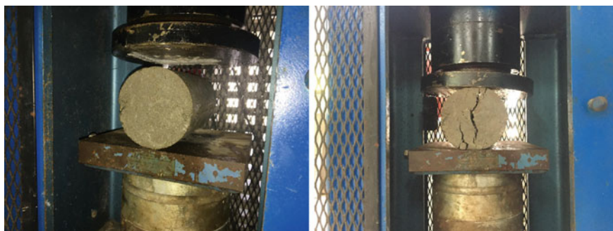
Fig. 4 Tensile strength test arrangement
