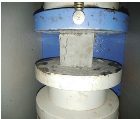
Fig. 3 Failure pattern of mortar cube testing in CTM
