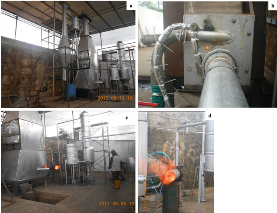
Fig. 7 Fabricated biochar plant at Gohagoda MSW disposal site (a) biochar plant, (b) biochar plant at operation (c), (d) producer gas flame from gasifier
