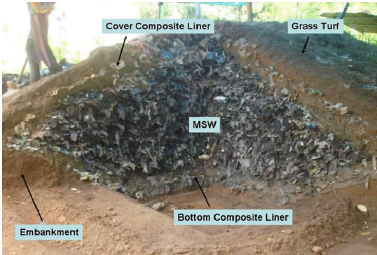
Fig. 14 Slicing through the landfill bioreactor profile. (Ecotech Lanka Ltd 2011)
