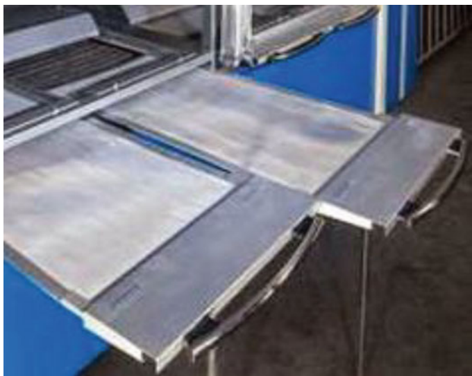
Fig. 49 Screens to filter lint
