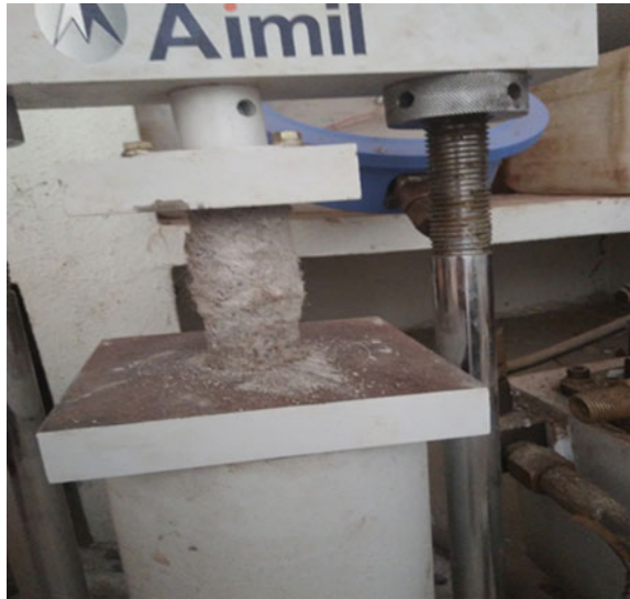
Fig. 5 Plastic in soil-cement sample failure
