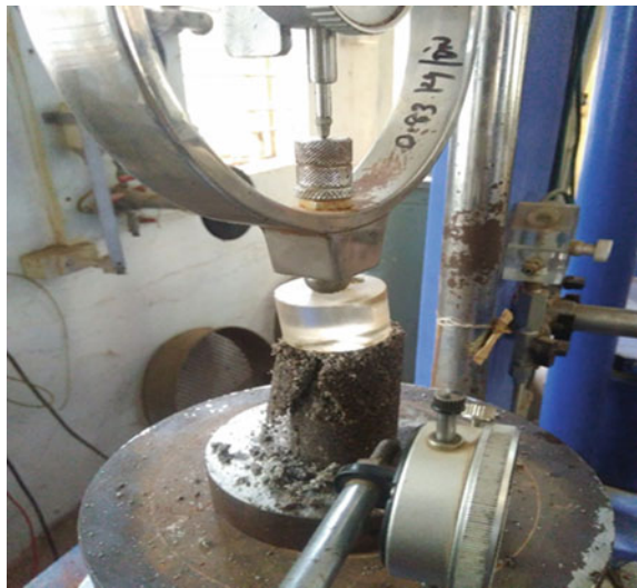
Fig. 4 Sand–plastic sample failure
