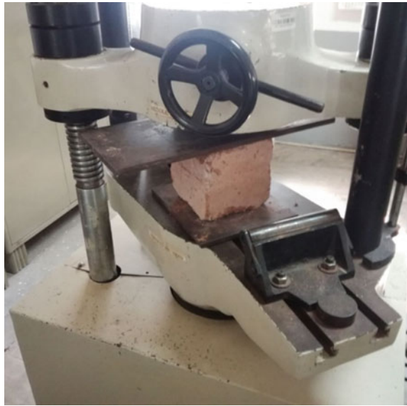
Fig. 7 Compressive testing on rammed earth cubes
