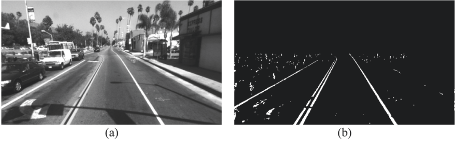
Fig. 2. (a) The grayscale image. (b) The result of feature image in binary.
