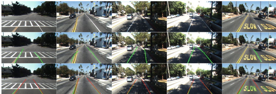
Fig. 5. Detection samples in Caltech Dataset. The first row is the origin image. The second row is result of Aly’s method. And the last row is ours, in where the green points are detected lines covered with features and the red lines are selected lane lines. (Color figure online)
