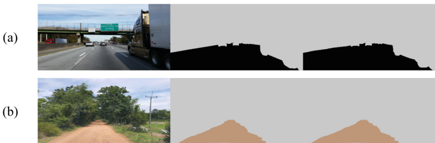
Fig. 4. Prediction result of 50 over-sampling model with Mapillary Vistas test dataset, the left column is the original image, the middle column is the GT, and the right column is the prediction: (a) Paved road prediction result. (b) Unpaved road prediction result.
