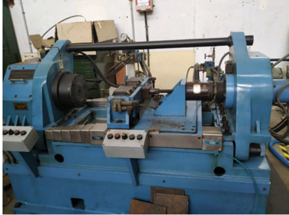
Fig. 1 Experimental set-up of friction welding process
