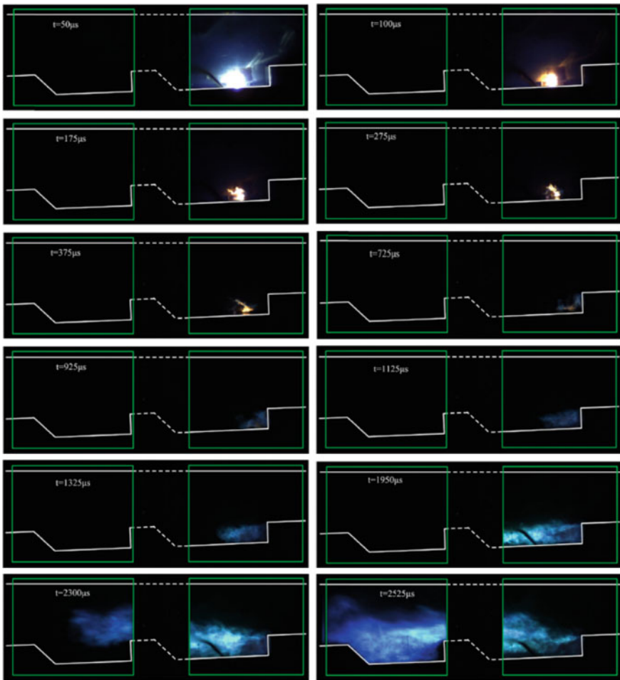
Fig. 4.7 High-speed images for evolution of the flame kernel induced by LIP ignition [6]
