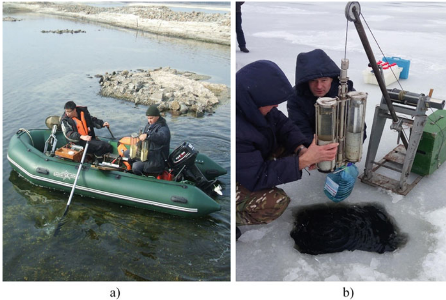
Fig. 8.5 Water sampling on the CP: (a) from boat; (b) from ice
