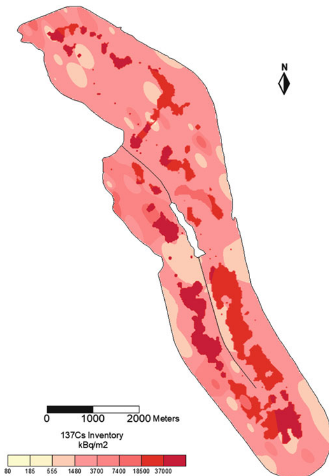
Fig. 8.26 Distribution of ^{137}\text{Cs} in the CP bottom sediments (modified after Voitsekhovych et al. 2013 using 2016 updated topography map)
