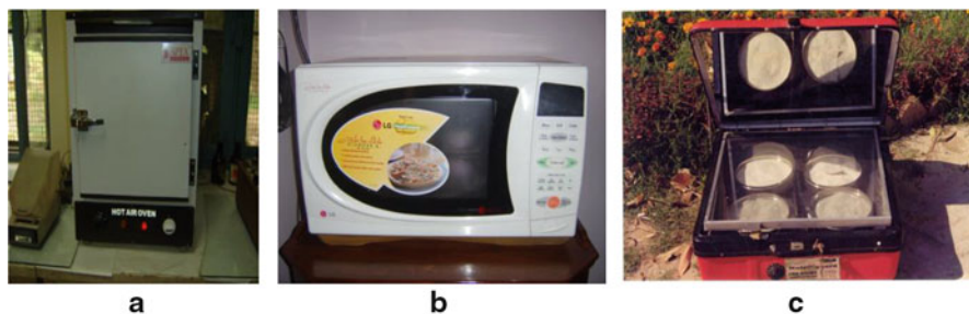
Fig. 1 Photographs of (a) cabinet dryer, (b) microwave oven dryer, (c) solar dryer
