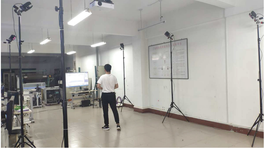
Fig. 1. Motion capture sites and markers. The NOKOV optical motion capture system used in the study consists of 6 optical motion cameras, markers, positioning rods, correction rods, data transmission equipment, upper computer.
