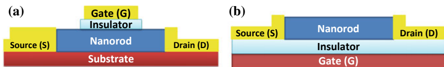
Fig. 10 Schematic diagram of top gate staggered structure (a) and bottom gate (inverted) staggered structure (b) of nanorod-based transistors
