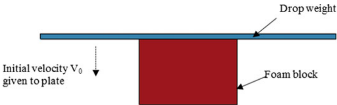
Fig. 5.4 Simulation of drop tower test using LS-DYNA
