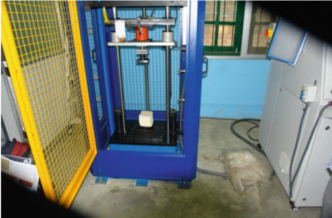
Fig. 5.1 Experimental setup for drop tower experiment on foam block of 150 mm × 150 mm × 100 mm
