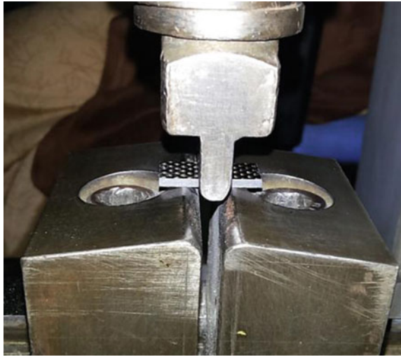
Fig. 18.5 ILSS test setup at UTM
