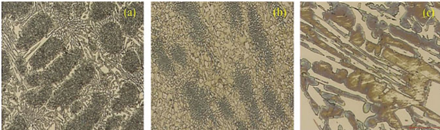
Fig. 25.5 Light microstructure of a HiCr, b HiCr5Mn and c HiCr10Mn samples at a magnification of 500 \times
