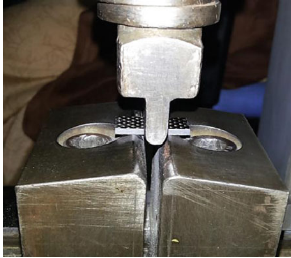
Fig. 18.5 ILSS test setup at UTM
