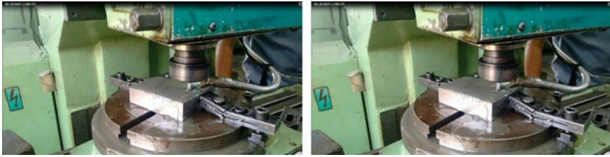
Fig. 21.4 Photographic view of milling machine with rotary table attachment for investigation
