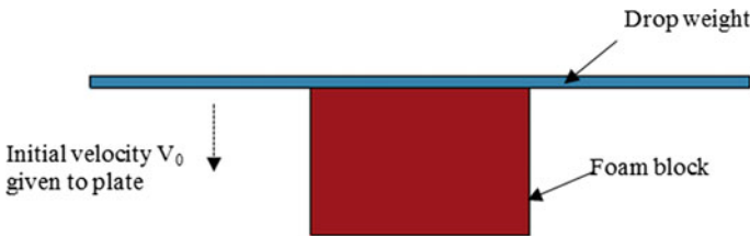
Fig. 5.4 Simulation of drop tower test using LS-DYNA
