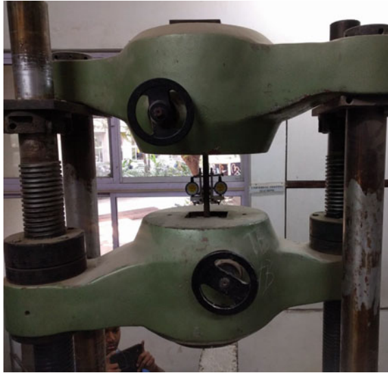
Fig. 15.4 Test setup for tension test on reinforcing bar
