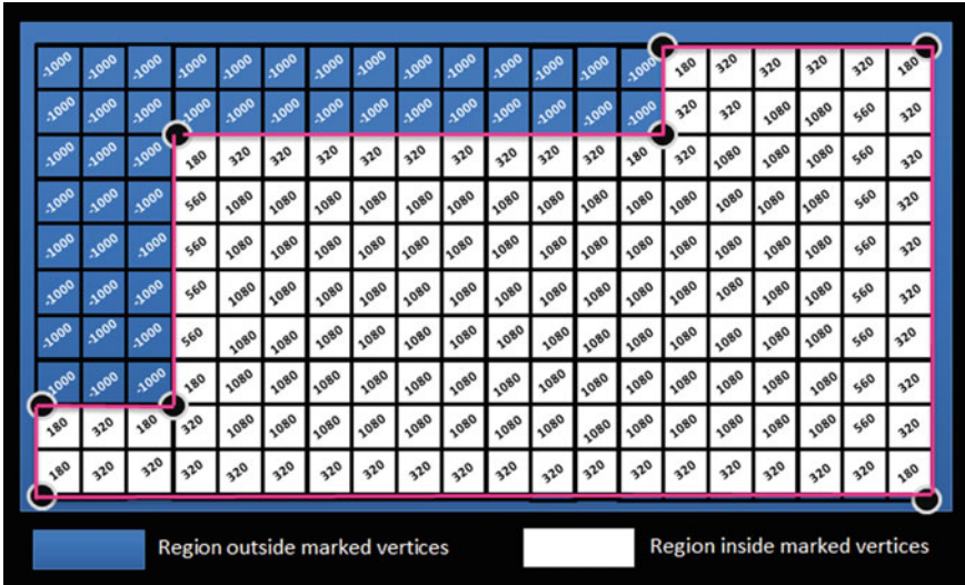
Fig. 6 Heatmap values generated for scanned rooftop
