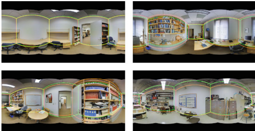
Fig. 4 Qualitative results (randomly sampled) on the Stanford 2D-3D annotation dataset. The Stanford dataset is more complex due to a more narrow field of view. Here, orange lines show IndoorNet’s layout prediction while green lines show the ground truth. Best viewed in color
