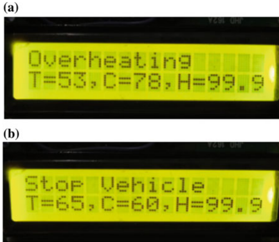
Fig. 4 Server messages to REV. T, C and H represent the temperature reading, SOC value and SOH value in both figures, respectively
