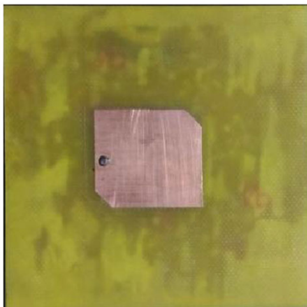
(b) Quad Frequency Fabricated antenna
