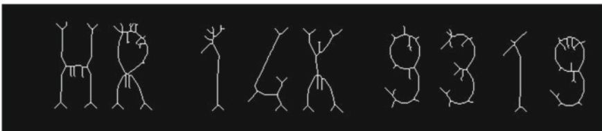
Fig. 4 Skeletal image of the license plate shown in Fig. 2
