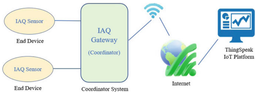
Fig. 2 IAQ monitoring system architecture
