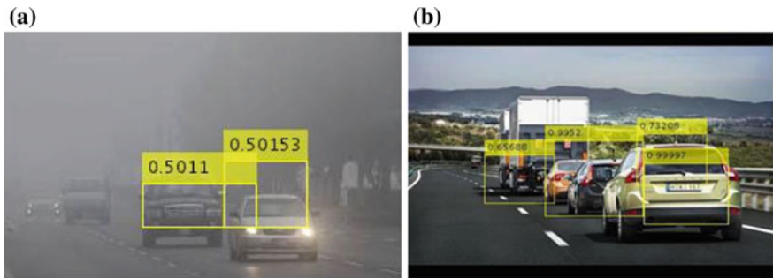
Fig. 3 a Detection in foggy weather; b detection in case of overlapping cars
