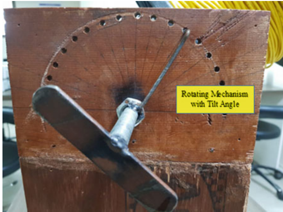
Fig. 6 Mechanism for manual measurement of tilt angle
