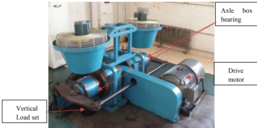
Fig. 2 Test rig of railway axle rolling bearings
