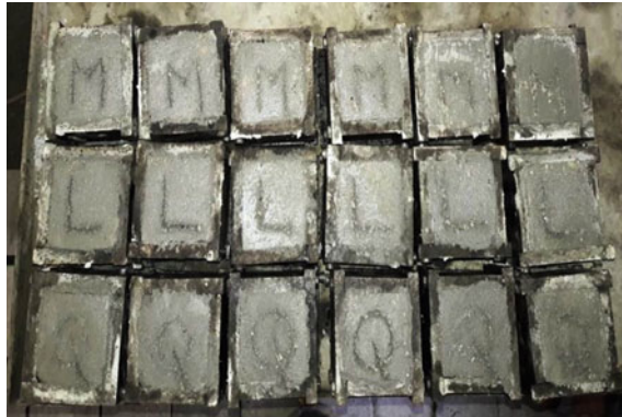
Fig. 4 Mortar cube of OPC, LC 3 and MC 3
