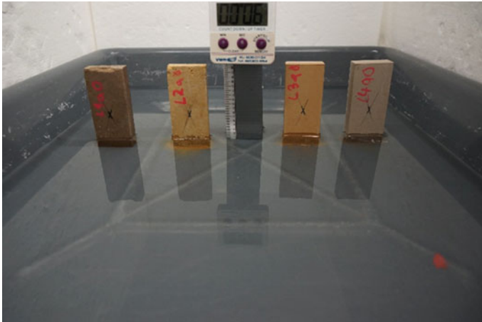
Fig. 5 Investigation setup for the determination of the water resistance
