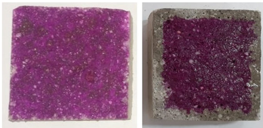
Fig. 1 Non-carbonated and carbonated specimens after 90 days
