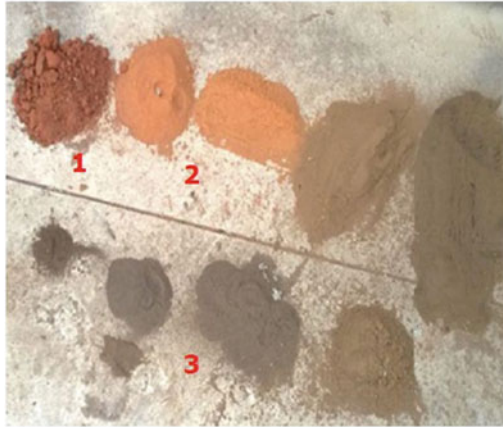
Fig. 3 (1) Raw material (2) Calcined material without Color control (3) Calcined material with color control process (Patent from FLSmidth)
