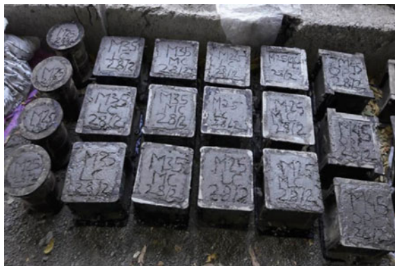
Fig. 5 Concrete cube and cylinder of OPC, LC 3 and MC 3
