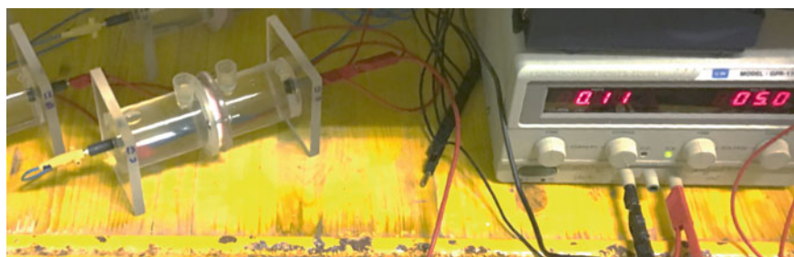
Fig. 1 The mini-migration set-up: the cement paste disc (33 mm diameter and 10 mm thickness) is placed between the upstream and downstream reservoirs in which electrodes provide a potential difference forcing the migration of chloride through the sample
