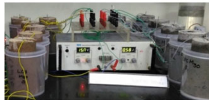
Fig. 3 Schematic diagram of impressed current corrosion test specimen and set-up
