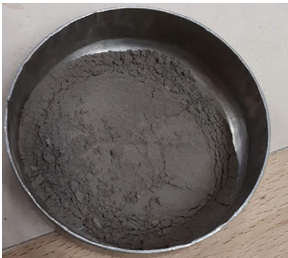
Fig. 6 Grinded pozzolan obtained in industrial trials
