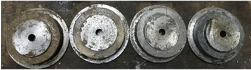
Fig. 3 Determination of restrained shrinkage in paste rings with the addition of illitic calcined clay
