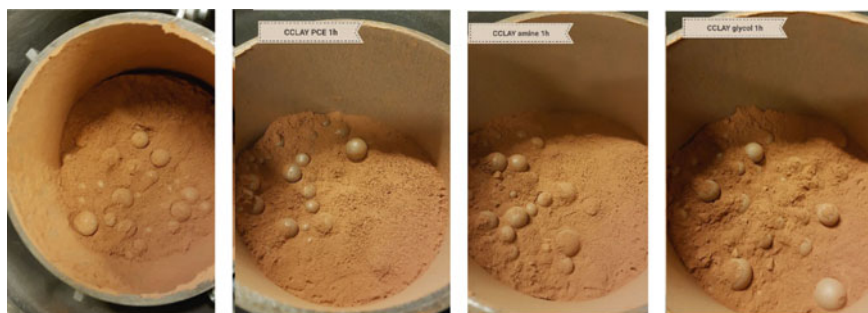
Fig. 1 Photographs of ground clay after 60 min incorporating (from left to right) no GA, PCE-based GA, Amine-based GA and Glycol-based GA
