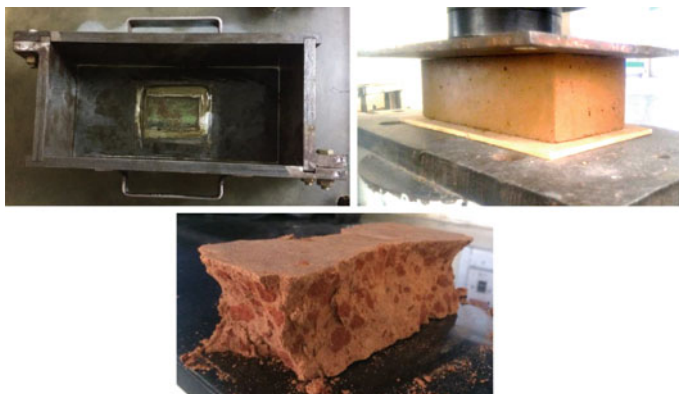
Fig. 5 Brick mould, compression test set-up and tested brick
