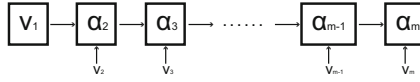
Fig. 2. The computing procedure of \alpha . The V_1 is the vector that is produced by the decoder corresponding to the first character of an inputted sentence. The value of \alpha_1 is set as V_1 . Except \alpha_1 , the solution of the value of \alpha_t at t step needs the V_t that is the vector corresponding to the character at t and the value of \alpha_{t-1} . The \alpha_m is the final result that can reflect the segmentation labels probability distribution of the whole sentence that is inputted to the model.
