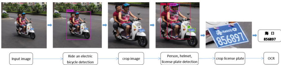
Fig. 1. Electric bicycle violation detection system. Our system mainly uses two technologies: (1) object detection with yolov3, (2) text recognition with the technology of chineseocr.
