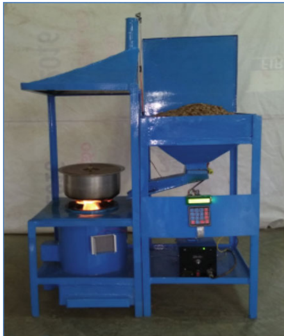
Fig. 7 Model-I (constructed) of biomass stove
