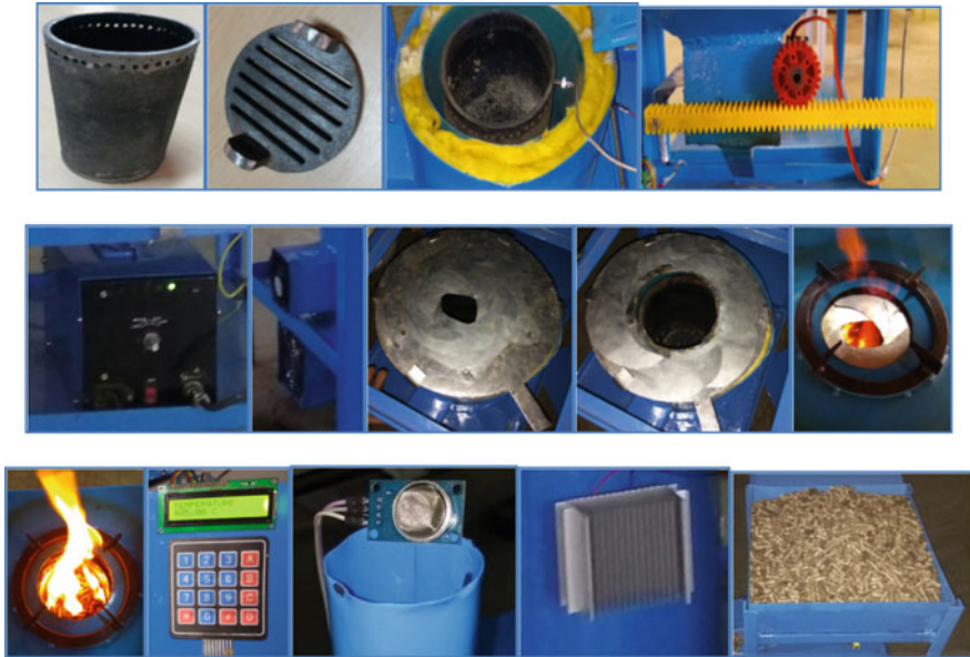
Fig. 8 Components of Model-I (from top left—combustion chamber, grate, thermal insulation and temperature sensor, rack and pinion mechanism, battery, primary and secondary fans, iris mechanism for closing and opening of aperture of combustion chamber, control panel, flue gas sensor, thermoelectric generator (TEG) module with heat sink, hopper and ashtray)
