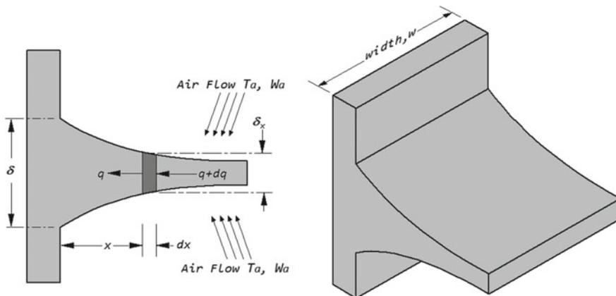
**Fig. 1** Schematic diagram of a completely wet straight longitudinal fin
