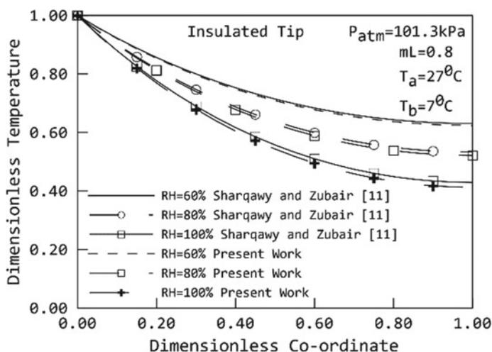
**Fig. 2** Comparison of normalized temperature distribution over fin length with that of obtained by Sharqawy and Zubair [11]
