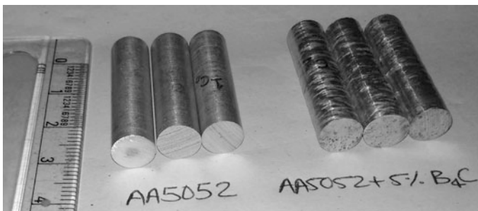
Fig. 3 Test samples after the abrasive wear test
