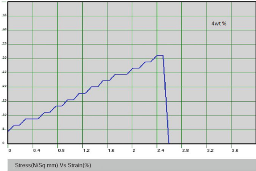
Fig. 5 Machine graph of tensile strength for 4 wt% eggshell-epoxy composite
