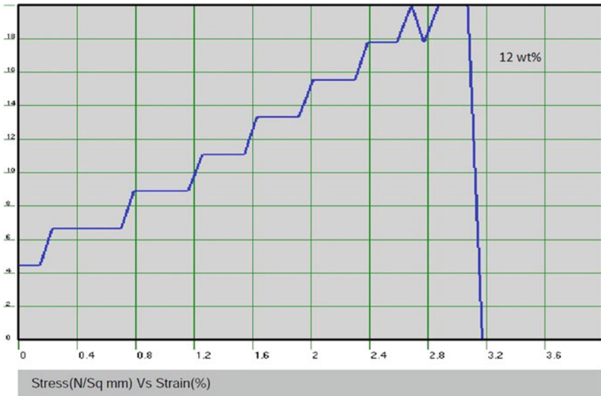
Fig. 7 Machine graph of tensile strength for 12 wt% eggshell-epoxy composite
