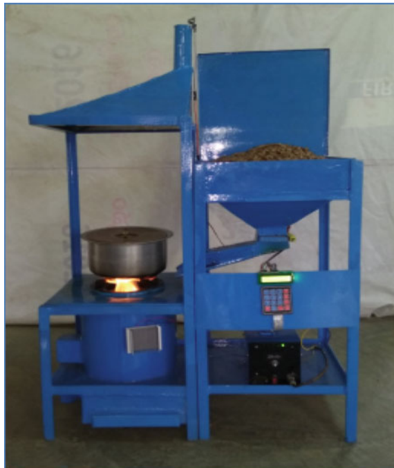
Fig. 7 Model-I (constructed) of biomass stove
