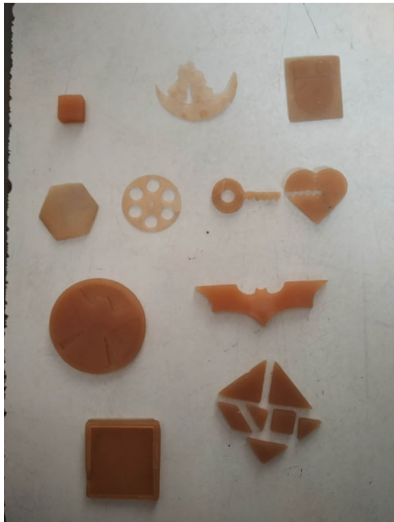
Fig. 5 Finished components made by our DLP 3D printer
