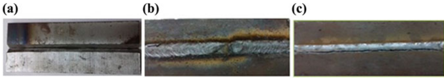
Fig. 1 a Base metal with V-groove before welding, b SMAW welded plate, c GMAW welded plate
