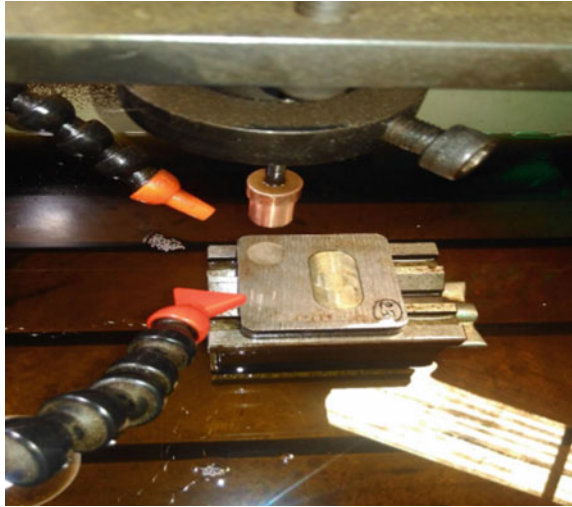
Fig. 2 Inconel-718 specimen after one of the trial runs on EDM
