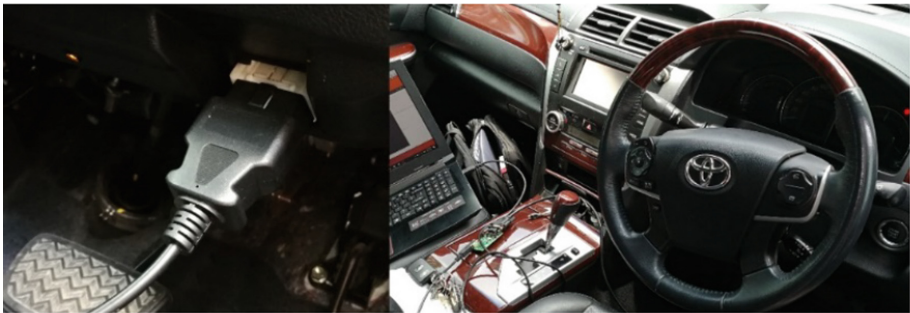
Fig. 2. Data acquisition setup through OBD-II port of Toyota Camry with CANTact device.
