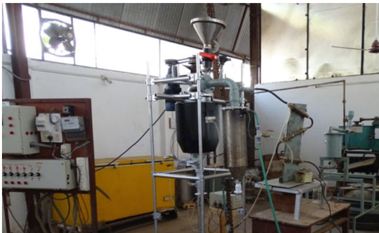
Fig. 19.1 Experimental setup to study the torrefaction of biomass at SPRERI
