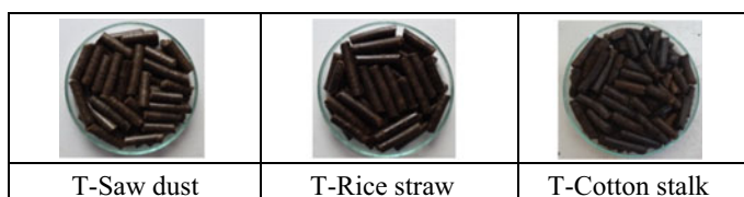
Fig. 19.4 Images of the 6 mm diameter pellets made from torrefied powered biomass materials at optimized conditions
