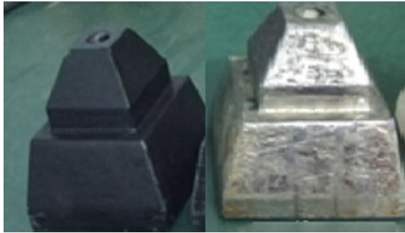
Fig. 41.7 Coated and electroplated FDM patterns
