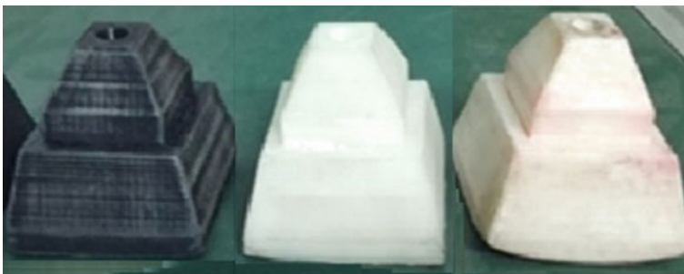
Fig. 41.4 FDM printed pattern
