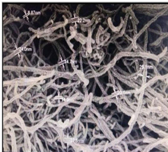
Fig. 5.3 SEM image of MWCNT
