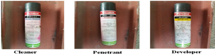
Fig. 3.6 Images of sprays used in dye penetration test
