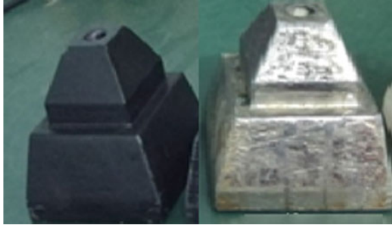
Fig. 41.7 Coated and electroplated FDM patterns
