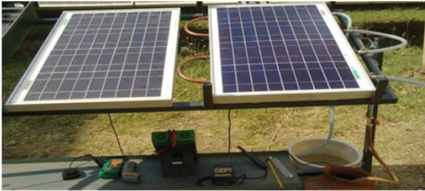
Fig. 47.5 Experimental setup of PV and PVT system [24]
