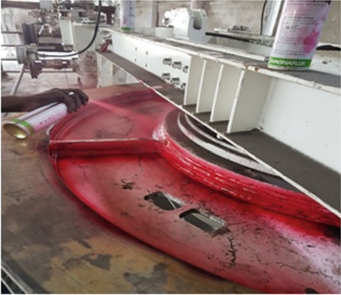
Fig. 3.7 Spraying penetrant on drive sheave
