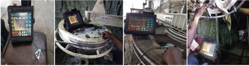
Fig. 3.4 Photographs of conducting ultrasonic flaw detection of MRCL
