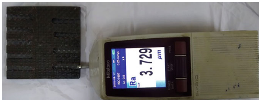
Fig. 49.3 Surface roughness measurement setup
