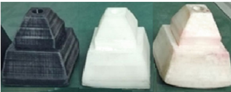
Fig. 41.4 FDM printed pattern
