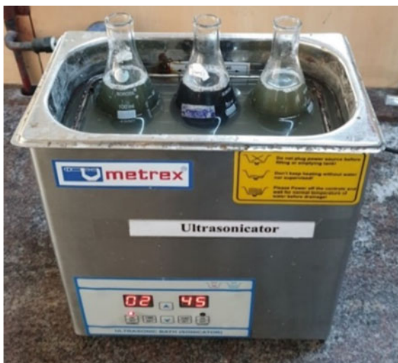
Fig. 5.6 Ultrasonicator used for homogeneous mixing
