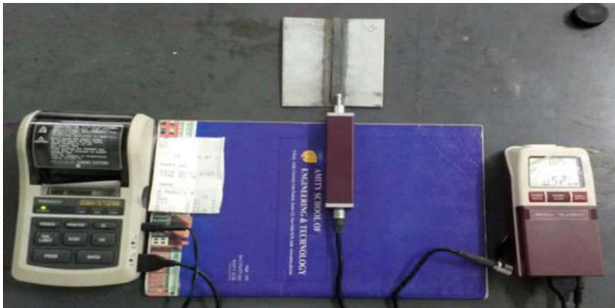
Fig. 65.4 Surface roughness measurement-TR 200 (calibrated with least count: 0.02 \mu\text{m} )
