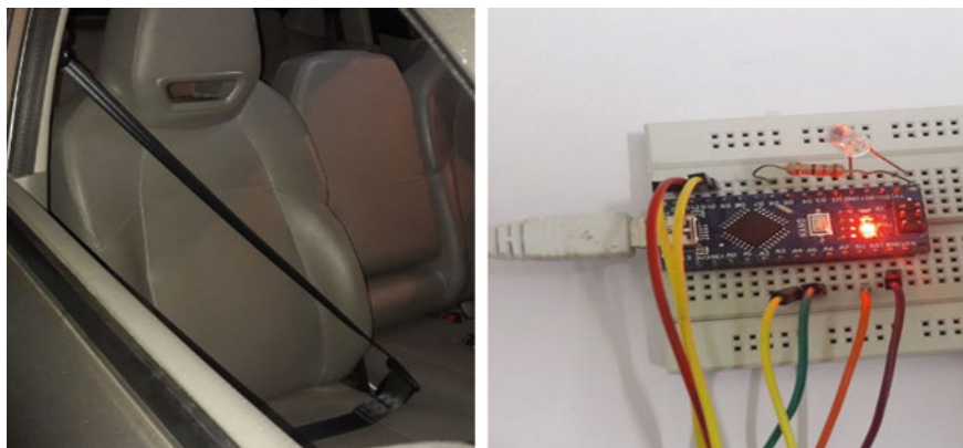
Fig. 12 Seatbelt locked in but no driver present between seat and seatbelt. Therefore, ignition command is not given to the ECU (If seatbelt is not locked in, same results are obtained)
