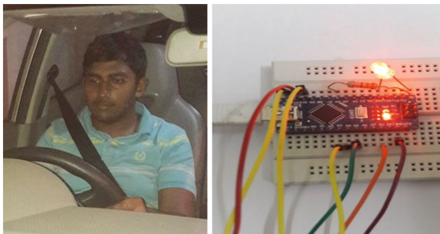
Fig. 13 Seatbelt locked in and driver present between seat and seatbelt. Therefore, ignition command is given to the ECU, represented by glowing LED
