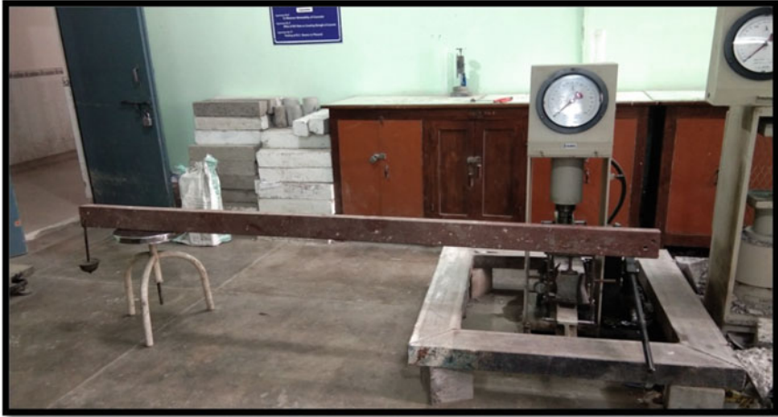
Fig. 10 Experimental set-up for combined test flexural and torsion
