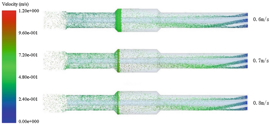
Fig. 3. Particle distribution map after 10 s simulation time with different velocity under 45-degree angle expansion
