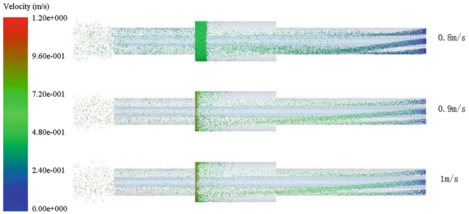
Fig. 2. Particle distribution map after 10 s simulation time with different velocity under right-angle expansion
