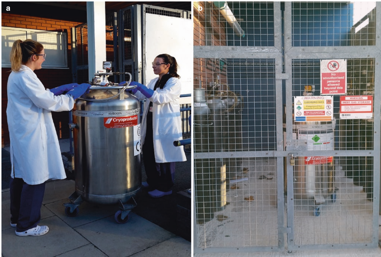
Fig. 65.2 (a) Clinic staff moving a bulk LN2 tank between the cryobank and a secure outdoor storage area (b) which can be accessed by the LN2 supply company. (Courtesy of the Knutsford Hewitt Fertility Centre, Liverpool Women's NHS Foundation Trust, Liverpool, UK)
