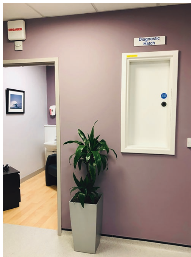
Fig. 64.5 Hatch for handing over semen samples. The hatch should be close to the production room to ensure the sample is passed to the andrologist immediately after production. Image courtesy of the Bristol Centre for Reproductive Medicine, Bristol, UK
