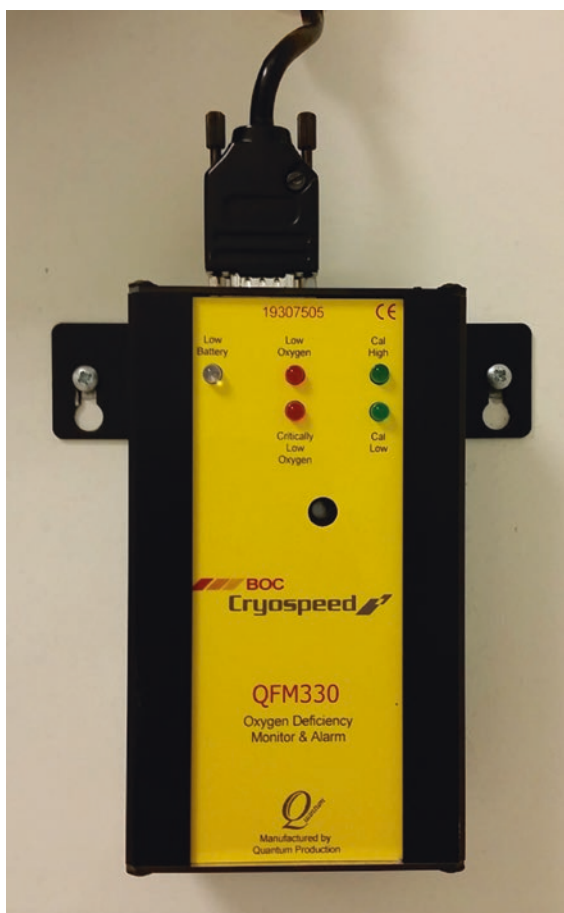
Fig. 65.3 An example of an oxygen monitoring device that can be used within the cryobank to detect low atmospheric oxygen. (Courtesy of the Knutsford Hewitt Fertility Centre, Liverpool Women's NHS Foundation Trust, Liverpool, UK)
