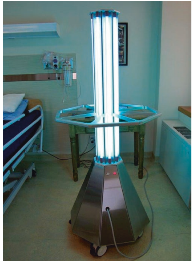
Fig. 75.3 Mobile UV unit for whole room surface disinfection. (Courtesy of Sanuvox Technologies, Montreal, Canada)
