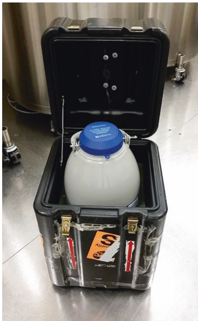
Fig. 65.8 A dry shipper. This specialist transport vessel is used to transport cryopreserved material between fertility clinics within the same country or internationally. (Courtesy of the Assisted Conception Service, Glasgow Royal Infirmary, Glasgow, UK)
