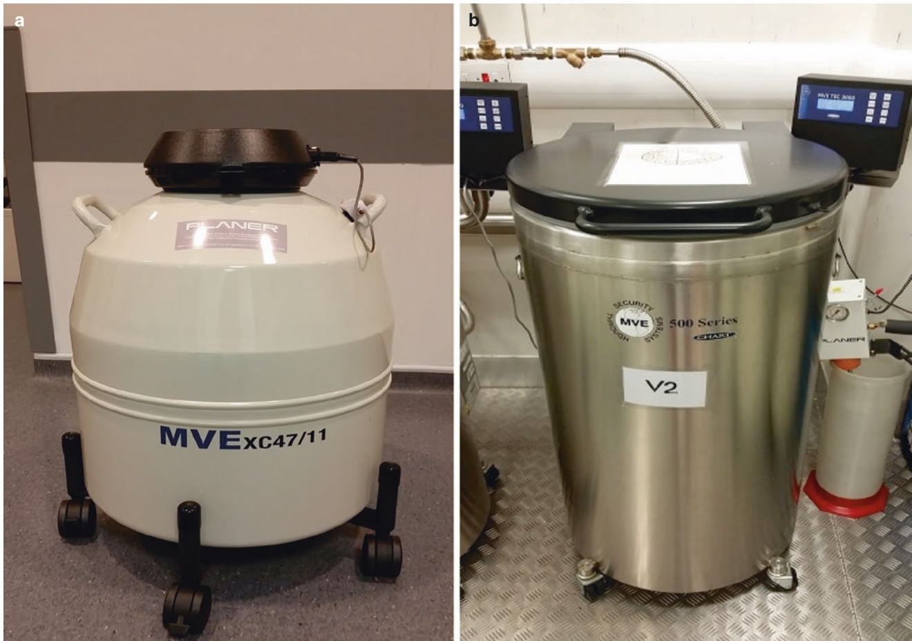
Fig. 65.5 (a) Example of a liquid-nitrogen based storage tank. (b) Example of vapour phase storage tank. (Courtesy of the Assisted Conception Service, Glasgow Royal Infirmary, Glasgow, UK)
