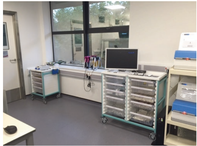
Fig. 74.3 Mobile furniture. Rather than using fixed fixtures and fittings, mobile units allow for laboratory redesign according to changing requirements. (Courtesy of the Knutsford Hewitt Fertility Center, Liverpool Women’s NHS Foundation Trust, Liverpool, UK)
