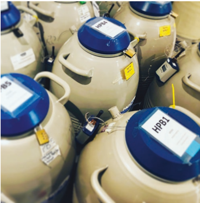
Fig. 64.1 Liquid nitrogen dewars in a cryobank. All dewars are individually padlocked and fitted with low level liquid nitrogen alarms to ensure samples are always maintained in a safe environment. Image courtesy of the Bristol Centre for Reproductive Medicine, Bristol, UK
