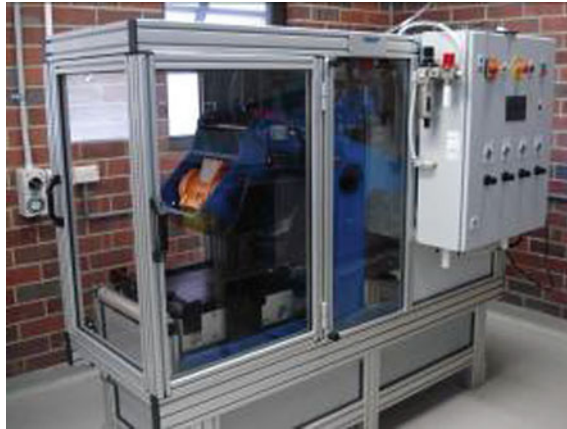
Fig. 2 Roller compactor used for manufacturing the CTB slabs
