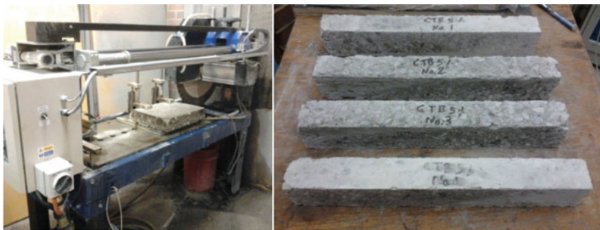
Fig. 3 Four prismatic beam specimens prepared from each compacted slab
