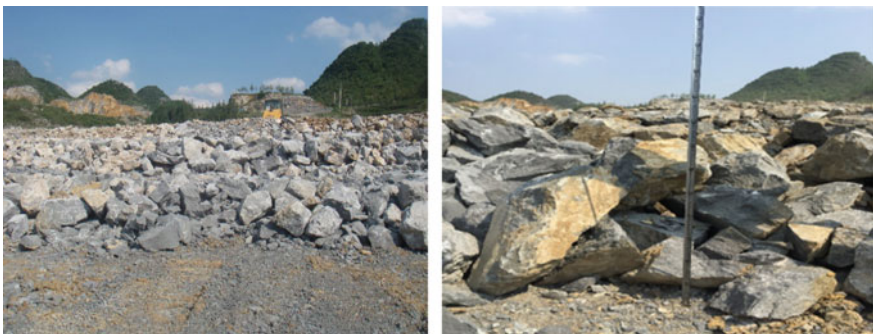
Fig. 1 The limestone for the embankment
