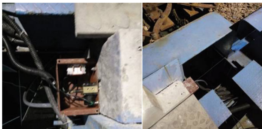
Fig. 9 Displacement sensor and its protective cover
