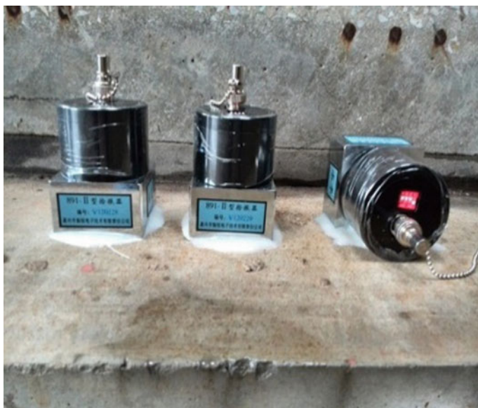
Fig. 5 Layout of the vibration sensors
