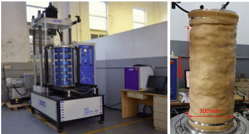
Fig. 4 Large diameter triaxial testing instrument and sample
