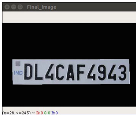
Fig. 3 Cropped out and enhanced number plate image* (resultant of the reference image) https://www.quora.com/How-are-number-plates-assigned-in-India
